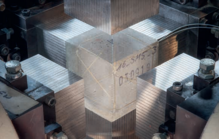
Test specimen with a fiber optic sensor in the triaxial testing machine in the Otto Mohr Laboratory of TU Dresden | Stefan Gröschel
