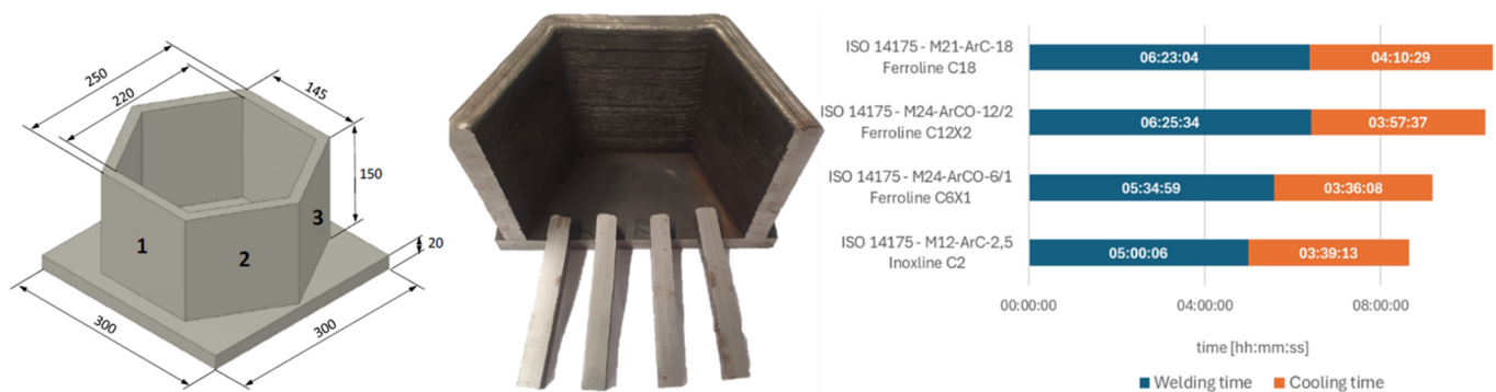
Fig. 1. Project with TU Ilmenau: WAAM component that has been printed four times with a different shielding gas; sample dimensions (left), macro cuts (middle), production time separated in welding and cooling time (right).
