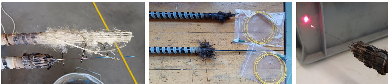
Fig. 1. Integrating optical fiber into pultruded BFRP bars (a) extracting the fiber from the bar; (b) connected pig tails (c) operational check.
