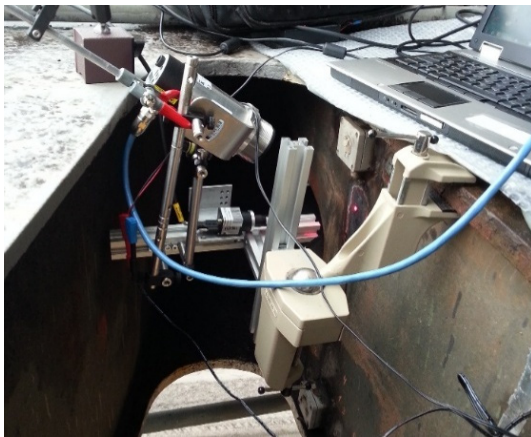
Fig. 4: Left: Placement of the LSP sensor system in the vicinity of the tension head of the overburden conveyor bridge. The measurement locations for the BN and LSP techniques are identical. Right: Total stress determined from the combined evaluation of both measurement methods during the extension of the bridge and the variation of its inclination angle. The BN technique was used to determine the initial value of the absolute stress, while the LSP method was applied to monitor the subsequent stress variations during the change in bridge position.
