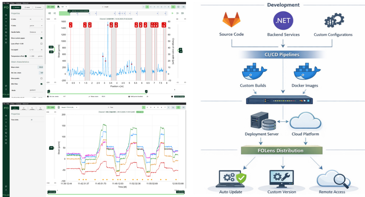
Fig. 1. FOlens desktop application for postprocessing of DFOS-data: (left top) length-domain analysis with strain results and crack width calculation, (left bottom) time-domain view showing strain evolution at selected gage positions during a load test, (right) FOlens system architecture.
